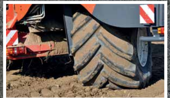
Super-wide rear wheel (1250/50 R32) with a tyre pressure of 1.4 bar.
