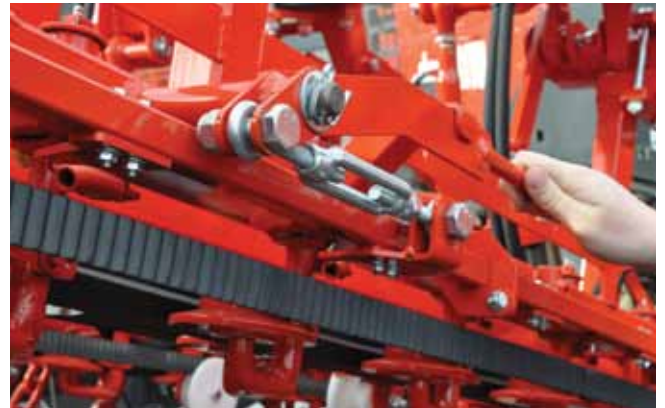
Via 1 handle per harvesting element all supporting pulleys of an element are tightened or loosened. This makes it much easier to replace a belt or remove blockages. (optional)
