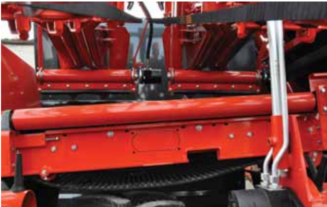
Rolls in front (option), under and behind the topping blades (standard) restrict losses and blockages to a minimum.
