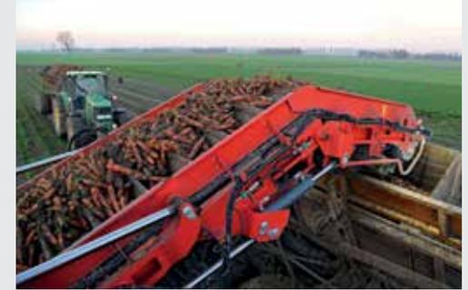
In order to harvest in an extra product-friendly manner, it is possible to have an optional hydraulically-adjustable fall breaker (C), a loading chute (A + B) or a container loader (D) (only for the ZKIIIs) at the end of the discharge elevator.
