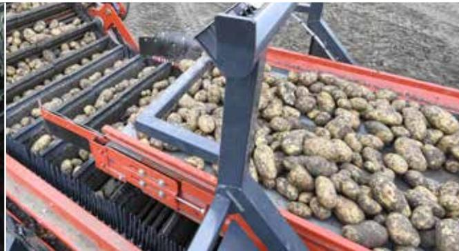
The inspection table is 90 cm wide. Long rubber flaps guide the product during transfer to the discharge elevator.
